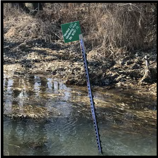
Trib 18787(1) Stream Gauge
